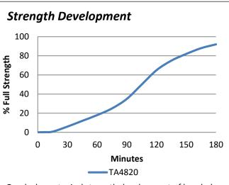
Graph shows typical strength development of bonded components at 23°C. Curing at higher or lower temperatures may affect cure speed.
