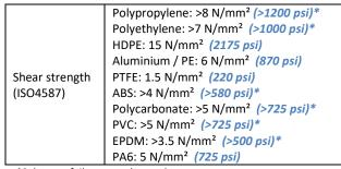
\*Substrate failure was observed.
