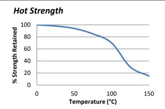
"Hot strength" shear strength tests performed on mild steel. Product fully cured at room temperature and conditioned to pull temperature for 30 minutes before testing.
