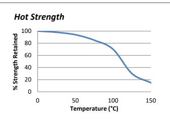
"Hot strength" shear strength tests performed on mild steel. Fully cured specimens conditioned to pull temperature for 30 minutes before testing at temperature. TA4246 can withstand higher temperatures for brief periods (such as for paint baking and wave soldering processes) providing the joint is not unduly stressed. The minimum temperature the cured adhesive can be exposed to is -40°C (-40°F) depending on the materials being bonded.
