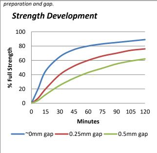
Graph shows typical strength development of bonded components at 23°C. Curing at higher or lower temperatures may affect cure speed.
