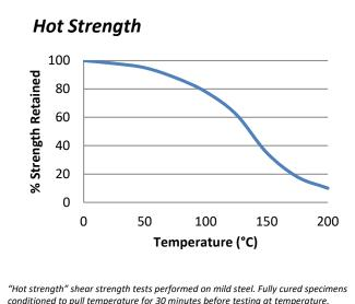
conditioned to pull temperature for 30 minutes before testing at temperature. TA4210 can withstand higher temperatures for brief periods (such as for paint baking and wave soldering processes) providing the joint is not unduly stressed. The minimum temperature the cured adhesive can be exposed to is -40°C (-40°F) depending on the materials being bonded.
