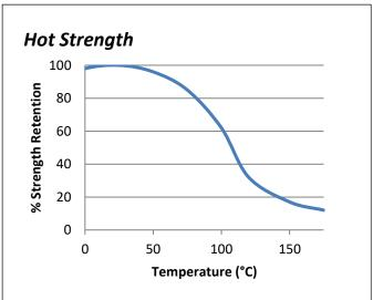
"Hot strength" shear strength tests performed on mild steel. Product fully cured at room temperature and conditioned to pull temperature for 30 minutes before testing.
