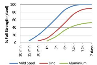
\*Cure times are typical at 23°C. Copper and its alloys will follow the faster cure while oxidised or passivated surfaces like stainless steel will tend towards the slower curve. Lower temperatures or large gaps will tend to extend the cure time. To reduce the cure time the use of Permabond A905, ASC10, or heat can be considered.
