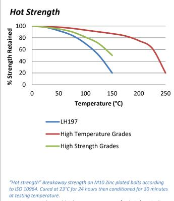
LH197 can withstand higher temperatures for brief periods (such as for paint baking and wave soldering processes) providing the joint is not unduly stressed. The minimum
