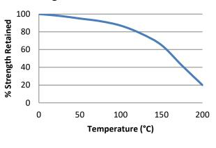
"Hot strength" Breakaway strength on M10 Zinc plated bolts according to ISO 10964. Cured at 23°C for 24 hours then conditioned for 30 minutes at testing temperature.
