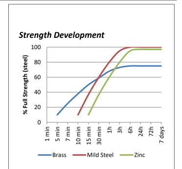
\*Cure times are typical at 23°C. Copper and its alloys will follow the faster cure while oxidised or passivated surfaces like stainless steel will tend towards the slower curve. Lower temperatures or large gaps will tend to extend the cure time. To reduce the cure time the use of
