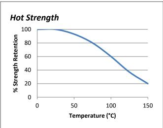
"Hot strenath" shear strenath tests performed on mild steel. Fully cured specimens conditioned to pull temperature for 30 minutes before testing at temperature.
