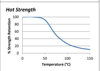
"Hot strength" shear strength tests performed on mild steel. Fully cured specimens conditioned to pull temperature for 30 minutes before testing at temperature. ET5364 can withstand higher temperatures for brief periods (such as for paint baking and wave soldering processes) providing the joint is not unduly stressed. The minimum temperature the cured adhesive can be exposed to is -40°C (-40°F) depending on the materials being bonded.
