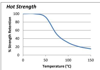
"Hot strength" shear strength tests performed on mild steel. Fully cured specimens conditioned to pull temperature for 30 minutes before testing at temperature. ET515 can withstand higher temperatures for brief periods (such as for paint baking and wave soldering processes) providing the joint is not unduly stressed. The minimum temperature the cured adhesive can be exposed to is -55°C (-65°F) depending on the materials being bonded.
