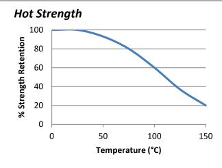
"Hot strenath" shear strenath tests performed on mild steel. Fully cured specimens conditioned to pull temperature for 30 minutes before testing at temperature.
