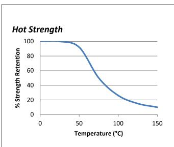
"Hot strength" shear strength tests performed on mild steel. Fully cured specimens conditioned to pull temperature for 30 minutes before testing at temperature.
