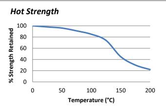
"Hot strength" shear strength tests performed on mild steel. Fully cured then conditioned to pull temperature for 30 minutes before testing.
