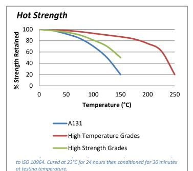
A131 can withstand higher temperatures for brief periods (such as for paint baking and wave soldering processes) providing the joint is not unduly stressed. The minimum temperature the cured adhesive can be exposed to is -55°C (-65°F) depending on the materials being bonded.
