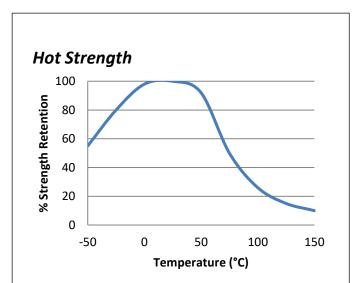
"Hot strength" shear strength tests performed on mild steel. 24hr cure at room temperature and conditioned to pull temperature for 30 minutes
