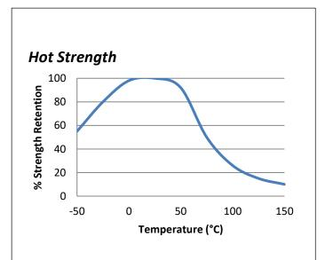
"Hot strength" shear strength tests performed on mild steel. 24hr cure at room temperature and conditioned to pull temperature for 30 minutes before testina.
