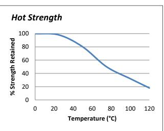
Fully cured lap shear specimens conditioned to pull temperature for 30 minutes before testing at temperature.
