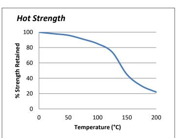
"Hot strength" shear strength tests performed on mild steel. Fully cured then conditioned to pull temperature for 30 minutes before testing. ES579 can withstand higher temperatures for brief periods (such as for paint baking and wave soldering processes) providing the joint is not unduly stressed. The minimum temperature the cured adhesive can be exposed to is -40°C (-40°F) depending on the materials being bonded.
