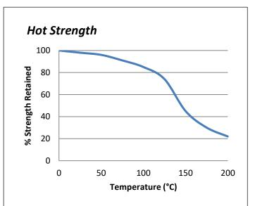
"Hot strength" shear strength tests performed on mild steel. Fully cured then conditioned to pull temperature for 30 minutes before testing. ES5748 can withstand higher temperatures for brief periods (such as for paint baking and wave soldering processes) providing the joint is not unduly stressed. The minimum temperature the cured adhesive can be exposed to is -40°C (-40°F) depending on the materials being bonded.
