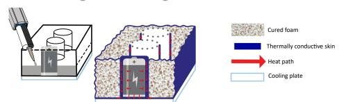
Permabond TC Filler expands during cure to form a lightweight foam surrounded by a highly thermally conductive skin.
