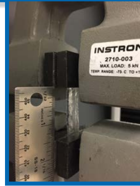
Cured 743 is stretched to over 4 times its length!
