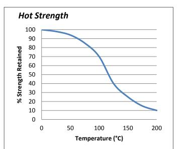
UV681 can withstand higher temperatures for brief periods (such as for paint baking and wave soldering processes) providing the joint is not unduly stressed. The minimum temperature the cured adhesive can be exposed to is -55°C (-67°F) depending on the materials being bonded.
