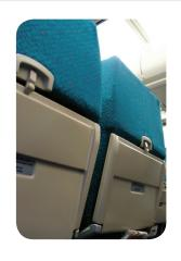
Application: Bonding aircraft seat trays Bonding ABS, plastic laminate and aluminium seat tray construction together. ET515 was selected due to its excellent impact and vibration resistance, quick cure and most importantly it doesn't attack any of the sensitive substrate materials.
