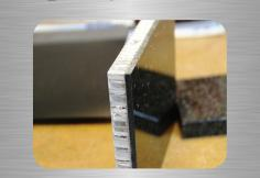
Bonding thin marble sections to honeycomb composite for use as worksurfaces in kitchens and bathrooms on yachts, motor homes, caravans and aeroplanes.
