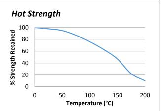
"Hot strength" shear strength tests performed on mild steel. Fully cured specimens conditioned to pull temperature for 30 minutes before testing at temperature. TA4592 can withstand higher temperatures for brief periods (such as for paint baking and wave soldering processes) providing the joint is not unduly stressed. The minimum temperature the cured adhesive can be exposed to is -55°C (-65°F) depending on the materials being bonded.
