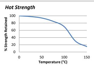
"Hot strength" shear strength tests performed on mild steel. Product fully cured at room temperature and conditioned to pull temperature for 30 minutes before testing.
