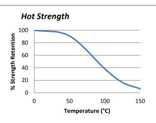
"Hot strength" shear strength tests performed on mild steel. Product fully cured at room temperature and conditioned to pull temperature for 30 minutes before testing.
