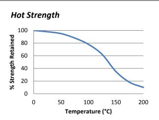
"Hot strength" shear strength tests performed on mild steel. Fully cured specimens conditioned to pull temperature for 30 minutes before testing at temperature. TA4210 can withstand higher temperatures for brief periods (such as for paint baking and wave soldering processes) providing the joint is not unduly stressed. The minimum temperature the cured adhesive can be exposed to is -40°C (-40°F) depending on the materials being bonded.
