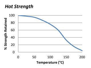
"Hot strength" shear strength tests performed on mild steel. Fully cured specimens conditioned to pull temperature for 30 minutes before testing at temperature. TA4204 can withstand higher temperatures for brief periods (such as for paint baking and wave soldering processes) providing the joint is not unduly stressed. The minimum temperature the cured adhesive can be exposed to is -40°C (-40°F) depending on the materials being bonded.
