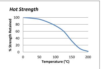
"Hot strength" shear strength tests performed on mild steel. Fully cured specimens conditioned to pull temperature for 30 minutes before testing at temperature. TA4202 can withstand higher temperatures for brief periods (such as for paint baking and wave soldering processes) providing the joint is not unduly stressed. The minimum temperature the cured adhesive can be exposed to is -40°C (-40°F) depending on the materials being bonded.
