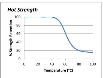
"Hot strength" shear strength tests performed on mild steel. Fully cured specimens conditioned to pull temperature for 30 minutes before testing at temperature.
