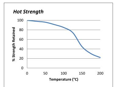
"Hot strength" shear strength tests performed on mild steel. Fully cured then conditioned to pull temperature for 30 minutes before testing. ES578 can withstand higher temperatures for brief periods (such as for paint baking and wave soldering processes) providing the joint is not unduly stressed. The minimum temperature the cured adhesive can be exposed to is -40°C (-40°F) depending on the materials being bonded.
