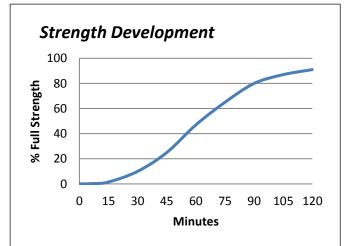
Graph shows typical strength development of bonded components at 23°C. Curing at higher or lower temperatures may affect cure speed.
