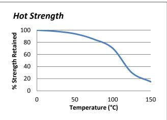
"Hot strength" shear strength tests performed on mild steel. Product fully cured at room temperature and conditioned to pull temperature for 30 minutes before testing.
