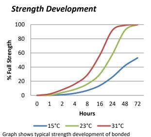
components. An increase of 8°C in temperature will halve the cure time. Lower temperatures will result in a slower cure time.
