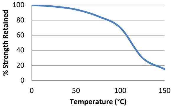
"Hot strength" shear strength tests performed on mild steel. Product fully cured at room temperature and conditioned to pull temperature for 30 minutes before testing.
