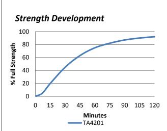
Graph shows typical strength development of bonded components at 23°C. An increase of 8°C in temperature will halve the cure time. Lower temperatures will result in a slower cure time.
