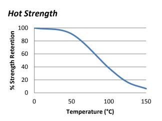
"Hot strength" shear strength tests performed on mild steel. Fully cured specimens conditioned to pull temperature for 30 minutes before testing at temperature. TA4201 can withstand higher temperatures for brief periods (such as for paint baking and wave soldering processes) providing the joint is not unduly stressed. The minimum temperature the cured adhesive can be exposed to is -40°C (-40°F) depending on the materials being bonded.
