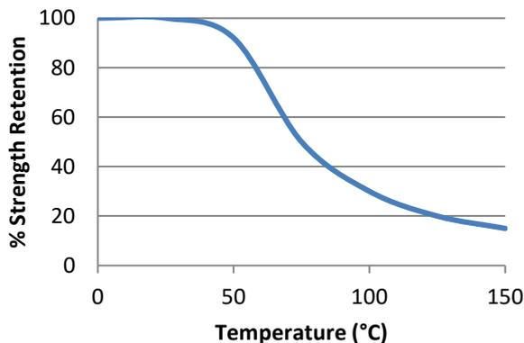
"Hot strength" shear strength tests performed on mild steel. Fully cured specimens conditioned to pull temperature for 30 minutes before testing at temperature. ET515 can withstand higher temperatures for brief periods (such as for paint baking and wave soldering processes) providing the joint is not unduly stressed. The minimum temperature the cured adhesive can be exposed to is -55°C (-65°F) depending on the materials being bonded.
